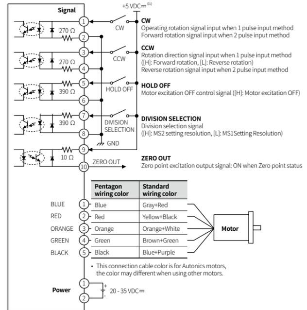
01) If the external signal input voltage is exceed the +5 VDC≒, connect a resistor at outside.
